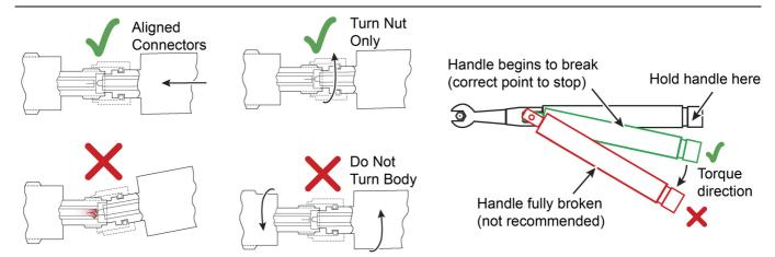
Carefully align the connectors so they are parallel to each other. The male connector center pin must slip concentrically into the contact fingers of the female connector.
