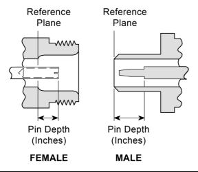
Figure 2-1. Pin Depth Example (N-Type Connector)
